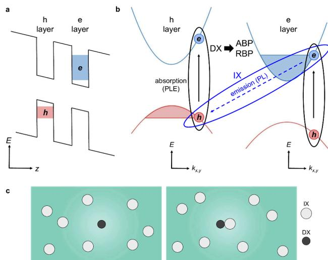
**Figure 1.** Diagram of an electron–hole bilayer. (a) Electrons (e) and holes (h) are confined in separated layers. (b) Absorption (PLE) and emission (PL) in bilayer heterostructure. Spatially indirect excitons (IXs) and direct excitons (DXs) are shown by the ovals. (c) Free DXs (left) and DX-IX bound states (right) interact with surrounding IXs and form repulsive and attractive Bose polarons (RBP and ABP).
