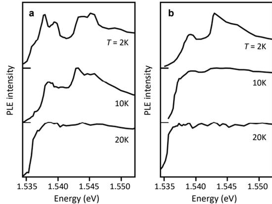
FIG. S2. PLE spectra at  $P_{\text{ex}} = 7.5$  (a) and 24 (b) mW at  $T = 2, 10,$  and 20 K. At high temperatures, the excitonic peaks vanish and the PLE spectrum becomes step-like as 2D density of states.
