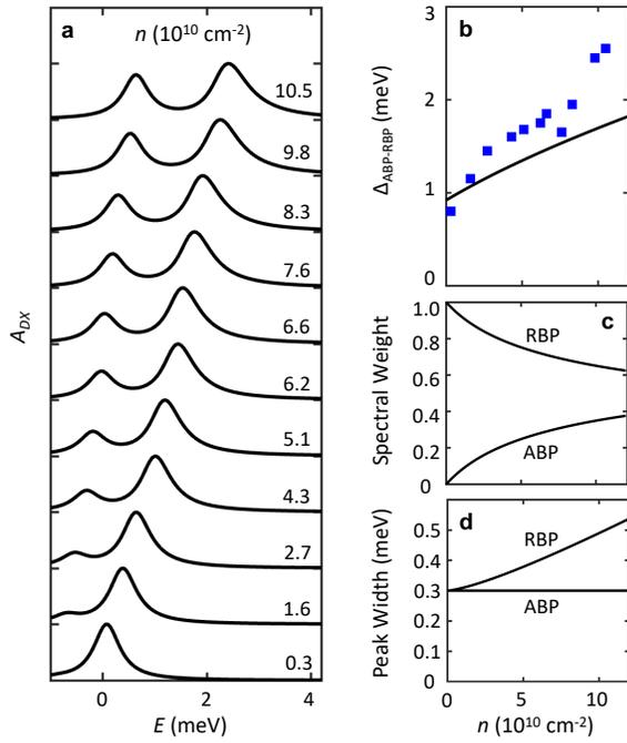
FIG. S5. (a) Calculated DX spectral function for different  $n$  using  $E_{XX} = (0.96 + 0.88)/2 = 0.92$  meV and damping  $\Gamma = 0.3$  meV. The lower-energy and higher-energy peaks correspond to the ABP and RBP, respectively. (b) The ABP-RBP energy splitting deduced from panel (a) (line). The squares are experimental data from Fig. 2 of the main text. (c) ABP and RBP spectral weight vs.  $n$ . (d) ABP and RBP peak width vs.  $n$ .
