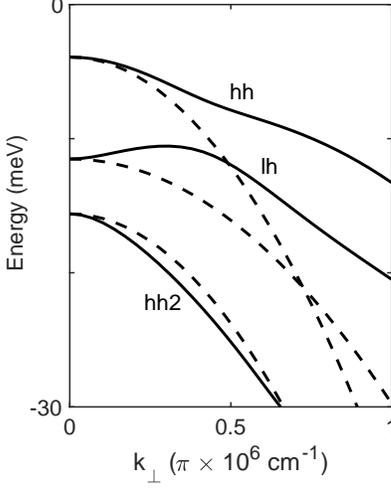
FIG. S3. In-plane dispersion  $\varepsilon_h(\mathbf{k}_\perp)$  for the first three hole subbands in units of meV. The dashed lines are the dispersions obtained by neglecting the coupling between heavy and light holes (the off-diagonal terms of  $H_h$ ).
